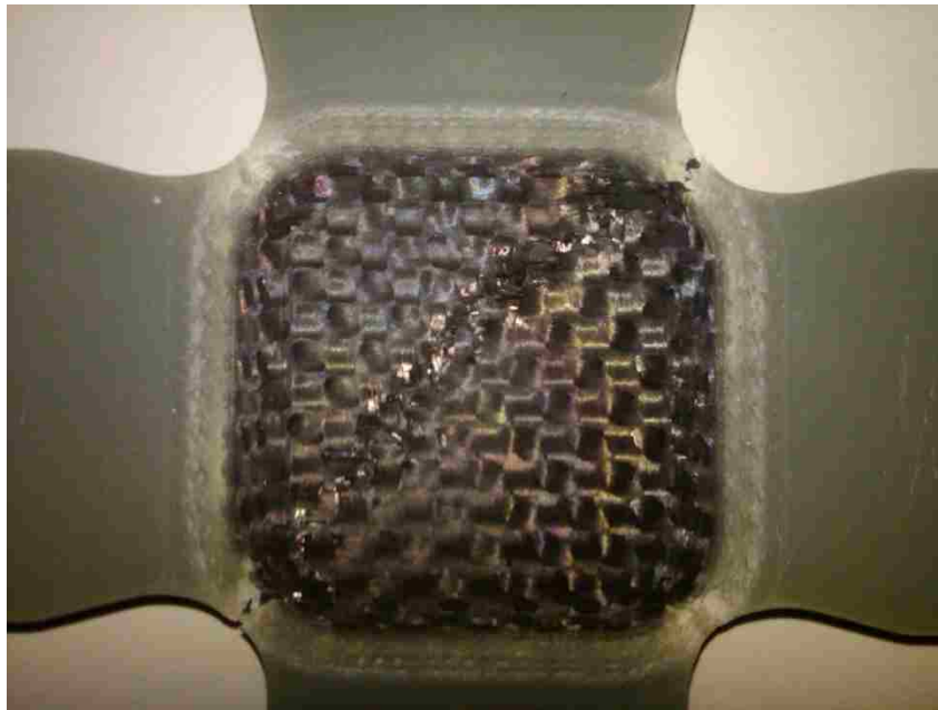
Figure 4.19: Adequate 45° failure mode for the Type II built-up specimen.
