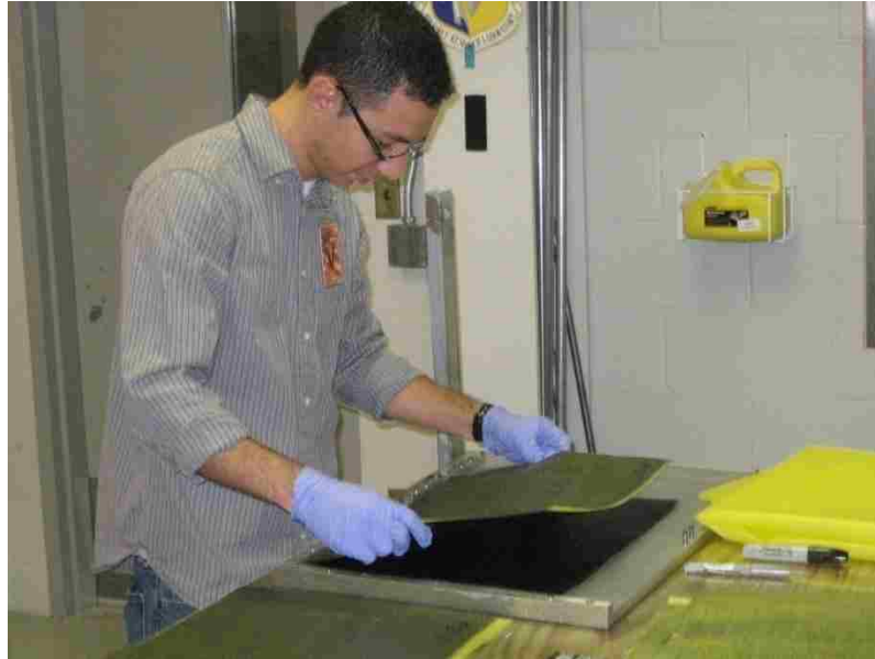
Figure 3.6: Lay-up process with aluminum jig for corner alignment.
