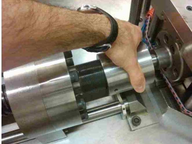
Figure 3.14: Tightening the cylindrical housing from the wedge grip arms to the screw drive.
