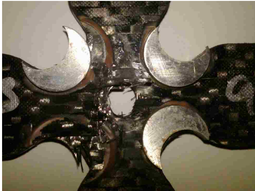
Figure 4.28: Center hole Type III shimmed specimen failure.
