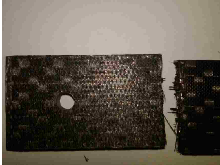
Figure 4.6: Untabbed uni-axial LAB failure in wedge grip.
