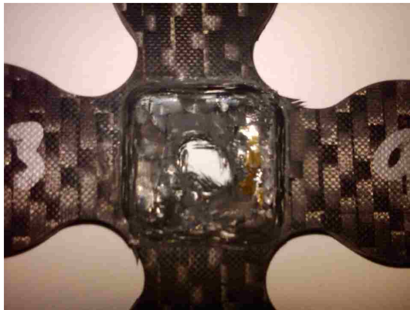
Figure 4.26: Center hole Type III control specimen failure.
